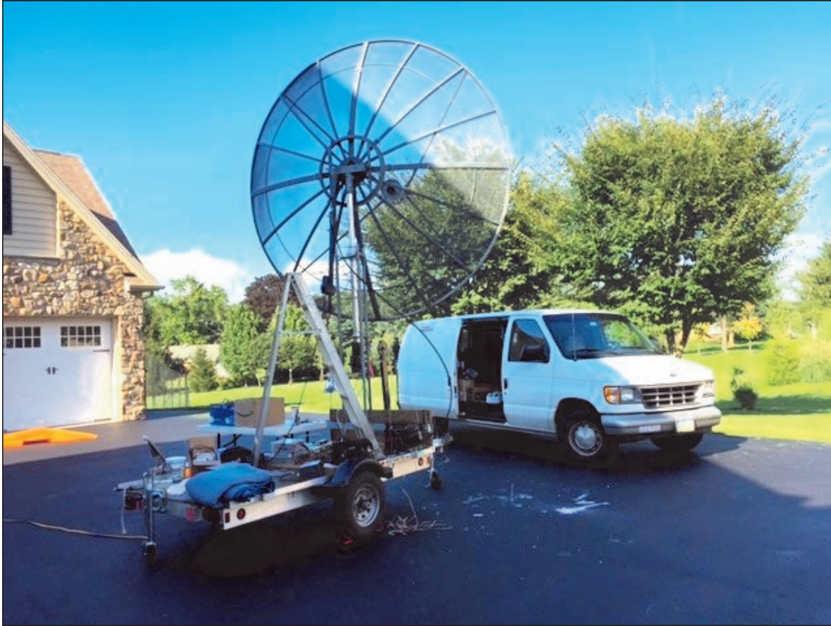
K1DS 13 CM rig set up for microwave EME contest.
